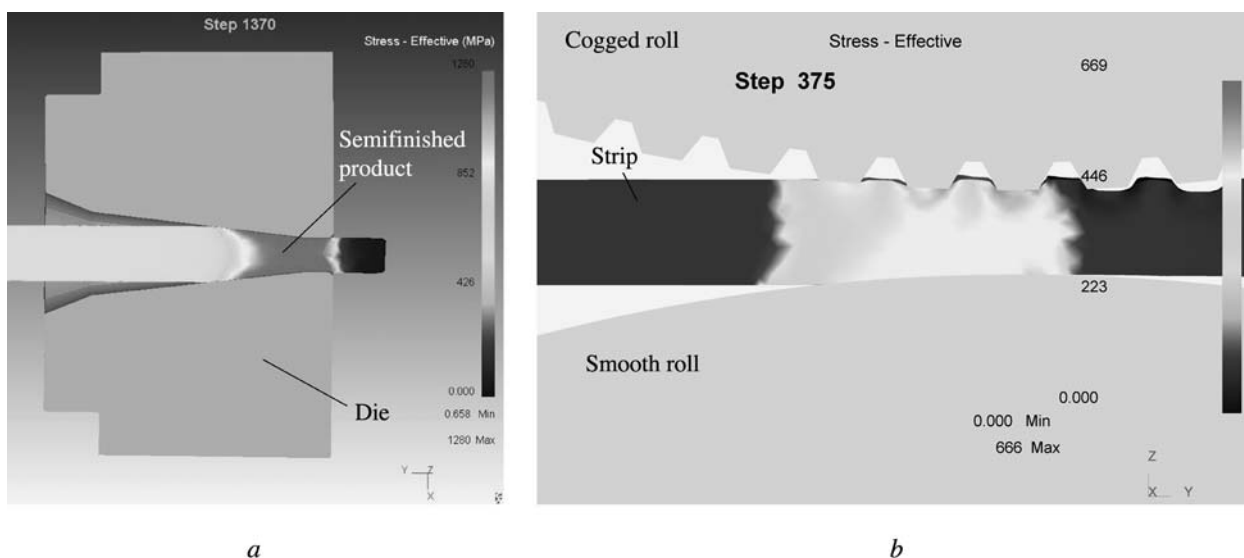
Fig. 3. Distribution of the equivalent stresses in a bar for a certain moment during its reduction on an AVS forging machine ( a ) and in a unilaterally finned strip rolled with a certain deformation increment ( b ).
