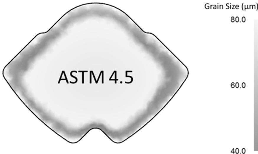
The new grain size model was initially studied on production 625 elbows forged on a hammer at U.S. Drop Forge. A cross-section of the forging showed the grain size through the center section. The actual production grain size in the center was ASTM 4. In the model, the predicted grain size was ASTM 4.5. The subsurface microstructure was predicted within 1.5 ASTM points. Another press forging at California Amforge was also tested with the new model. Grain size predictions were equally impressive.
