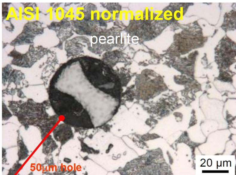
A workpiece was generated with 60% pearlite, 40% ferrite. Each phase was modeled as a discrete material. The flow stress was developed for each phase using a high rate compression test known as a Split Hopkinson Pressure Bar.
