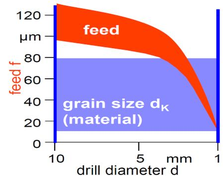
In micro-machining processes such as micro-drilling, holes may be smaller than 100µm. At this scale, chips are significantly smaller than grains and other microstructure features. For example, in a dual-phase steel, the pearlite regions can be up to three times harder than ferrite regions, and those regions are larger than the thickness of the chip.
