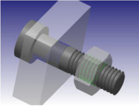
The bolted joint example studied the effect of vibration on preload in a bolted joint system. The graph (top right) shows the bolt loosening and preload reduction that resulted from plate vibration. DEFORM provides a framework for virtual testing by predicting response in complex systems.
