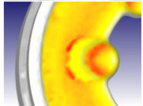
From a productivity standpoint, the production process offered room for improvement. The large deformation in the second station resulted in a high forging load. This prevented parts from being formed in stations 1 and 3 at the same time.
