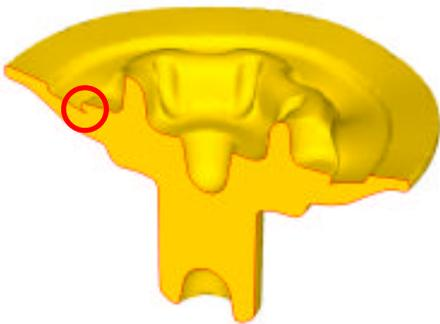
A modified "round" preform was developed to eliminate the lap. The simulation results were very promising. There were no defects, die fill was as expected and the die wear was reduced significantly.
