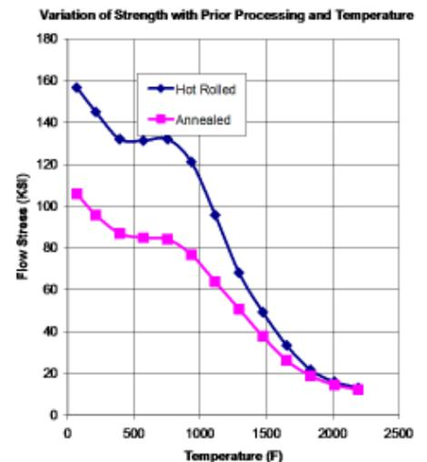
Because flow stress in cold forming is strongly history dependent, the best source of cold forming flow stress is testing the actual material to be formed, from the same supplier, and in the same anneal state that will be used in production. DEFORM support can provide a simple spreadsheet to convert yield and ultimate
