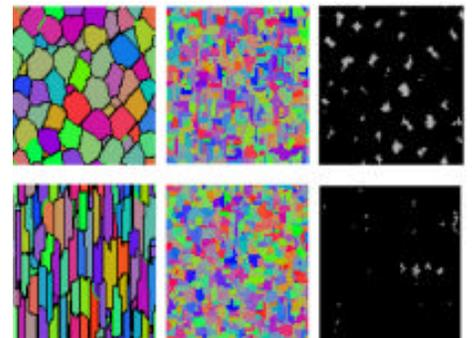
In this example, two different starting microstructures (equiaxed - top left & elongated - bottom left) are shown. The final microstructures are shown in the center. The unrecrystallized grains (gray) are shown on the right.
