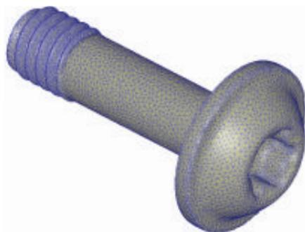
The FEM mesh is shown at the end of the thread rolling simulation.
