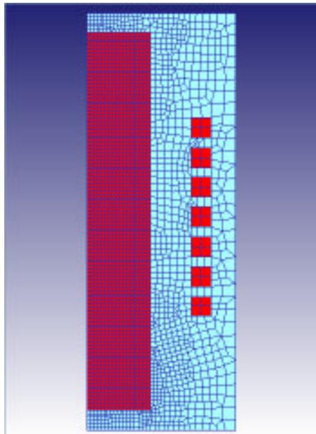
The DEFORM-2D axisymmetric problem set up, showing the common air object surrounding the 0.5" diameter waspaloy rod and the seven copper coil turns. All objects have an FEM mesh.
