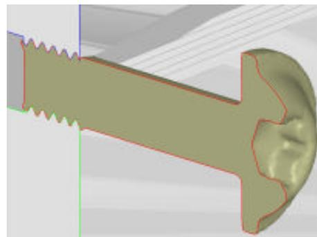
Slicing can be a useful tool when investigating thread unfill.
