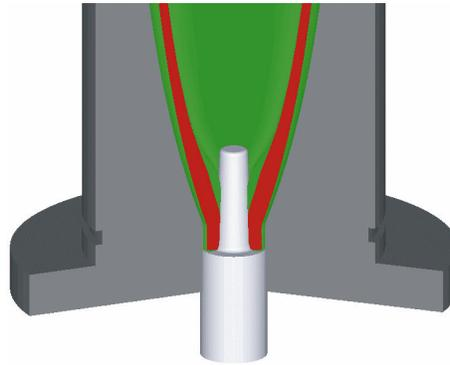
match a defect-free case. Extrusion stroke, pressure, temperature distribution and friction were varied to reproduce the observed defects. At the end of the project, the root cause of each forging-related defect was determined.
