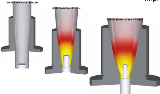
General Dynamics reported a range of frequent production problems. These included underfill in the nose, bulging on the outside diameter, inadequate blending, surface cracking, and excessive die wear. The nose underfill is shown (top center) with red being the underfilled condition.
